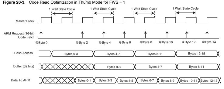
Note: When FWS is equal to 1, in case of sequential reads, all the accesses are performed in a single-cycle access (except for the first one).
