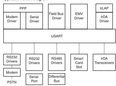
Figure 31-2. Application Block Diagram
