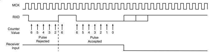
Figure 31-25. IrDA Demodulator Operations
