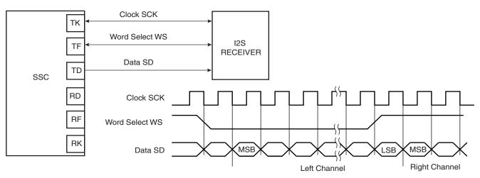
Figure 30-18. Codec Application Block Diagram
