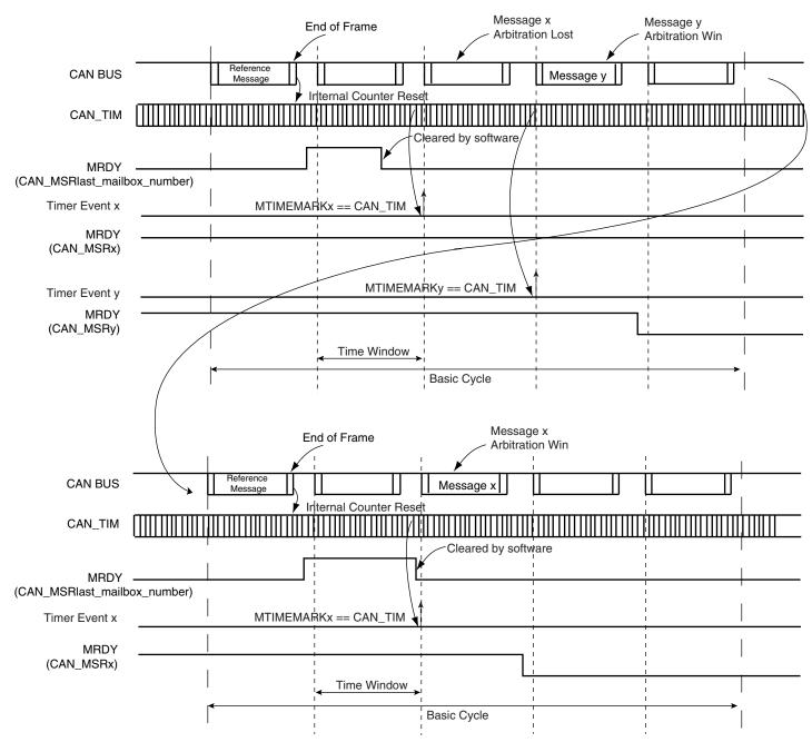
Figure 38-21. Time Triggered Operations
