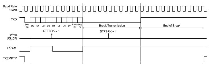
Figure 31-16. Break Transmission
