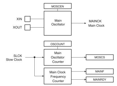
Figure 25-1. Main Oscillator Block Diagram
