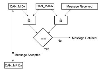
Figure 38-3. Message Acceptance Procedure
