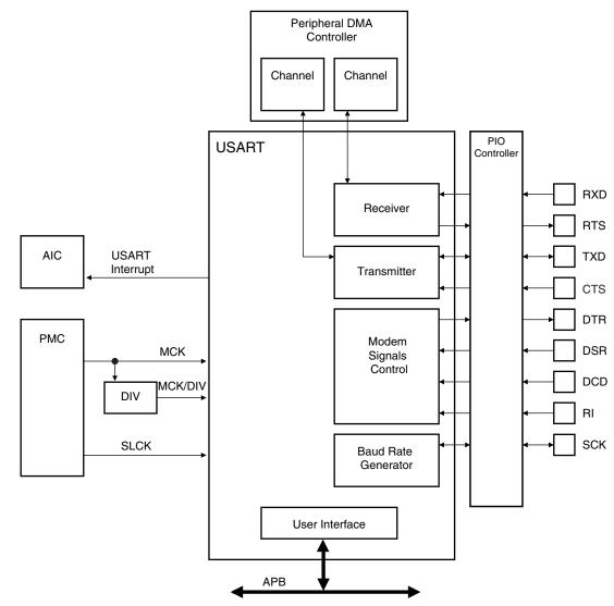
Figure 31-1. USART Block Diagram
