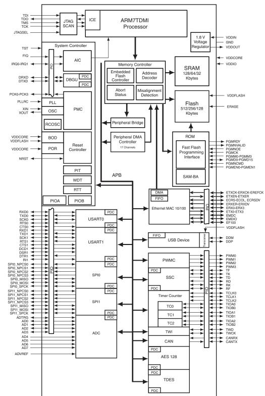
Figure 2-1. AT91SAM7XC512/256/128 Block Diagram
