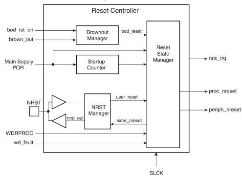
Figure 13-1. Reset Controller Block Diagram
