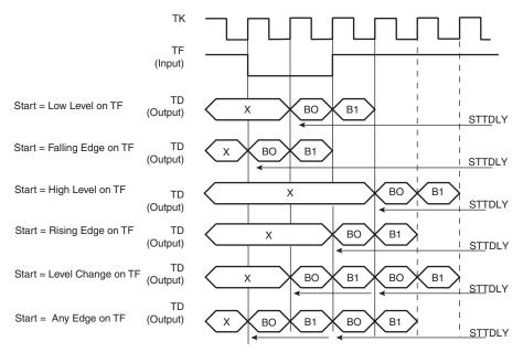
Figure 30-11. Receive Pulse/Edge Start Modes
