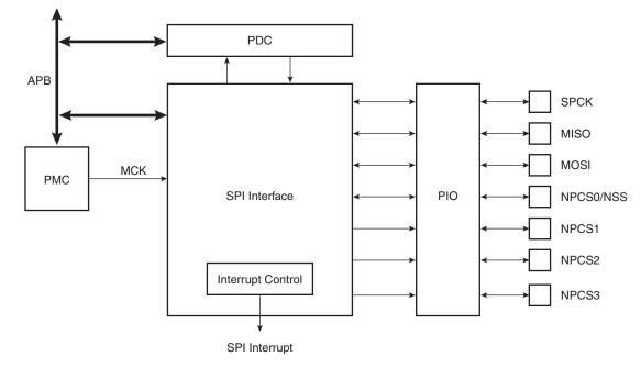
Figure 28-1. Block Diagram
