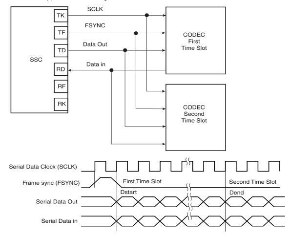
Figure 30-19. Time Slot Application Block Diagram
