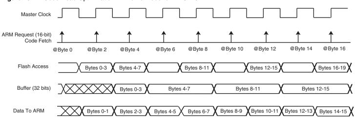
Figure 20-2. Code Read Optimization in Thumb Mode for FWS = 0
