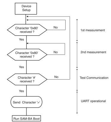
Once the communication interface is identified, the application runs in an infinite loop waiting for different commands as in Table 22-1.
