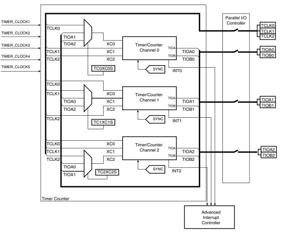
Figure 32-1. Timer Counter Block Diagram
