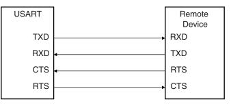
Figure 31-17. Connection with a Remote Device for Hardware Handshaking
