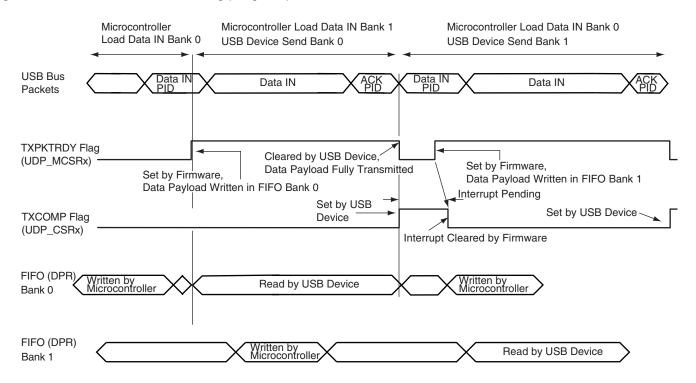
Figure 34-8. Data IN Transfer for Ping-pong Endpoint
