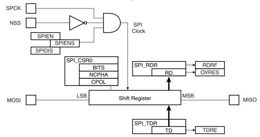
Figure 28-9. Slave Mode Functional Block Diagram
