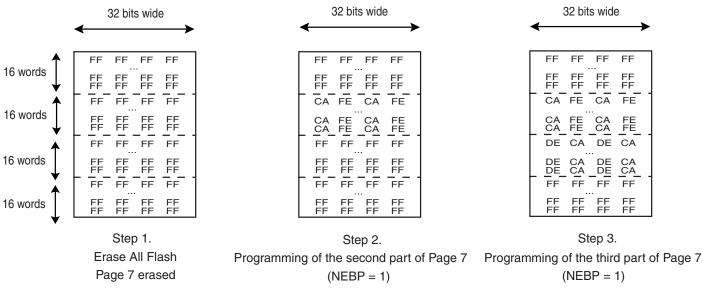
After programming, the page (the whole lock region) can be locked to prevent miscellaneous write or erase sequences. The lock bit can be automatically set after page programming using WPL.
