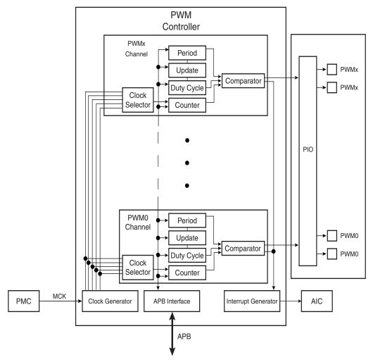
Figure 33-1. Pulse Width Modulation Controller Block Diagram
