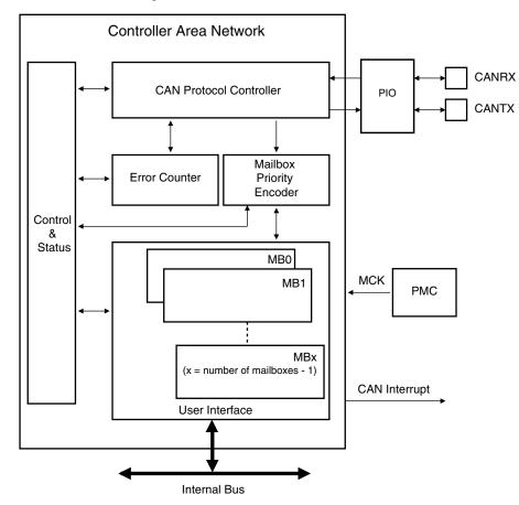
Figure 38-1. CAN Block Diagram
