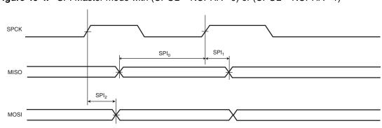
**Figure 40-4.** SPI Master mode with (CPOL = NCPHA =0) or (CPOL = NCPHA =1)
