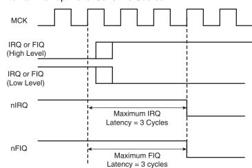
Figure 24-7. External Interrupt Level Sensitive Source
