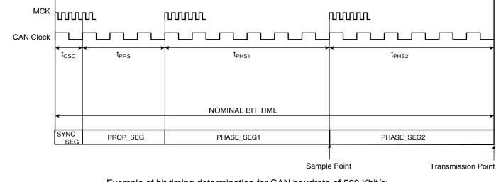
Figure 38-5. CAN Bit Timing
