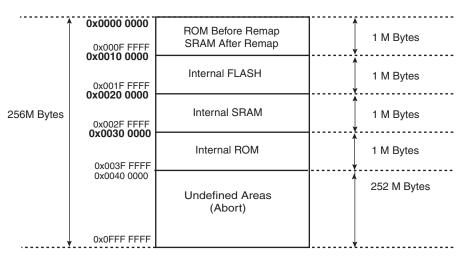
Figure 8-2. Internal Memory Mapping with GPNVM Bit 2 = 0 (default)
